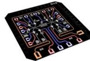
Figure 940: Alibaba's 11 qubit processor.
