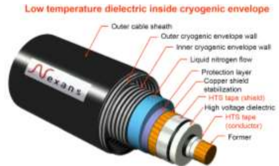
Figure 114: Nexans superconducting cable.
