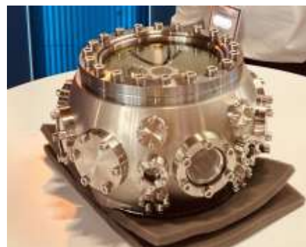
Figure 428: a vacuum chamber from Pasqal, which contains a MOT.
