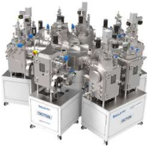
Figure 562: two examples of such cluster tools, on the left with a Kurt Lesker OCTOS Automated Thin Film Deposition Cluster Tool ( source ) and on the right an Applied Materials Endura Clover MRAM PVD System ( source ).
