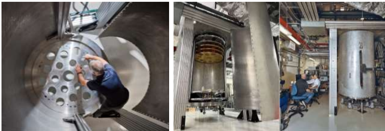
Figure 321: IBM's giant Goldeneye dilution refrigerator, which is currently put on hold. Source: IBM.
