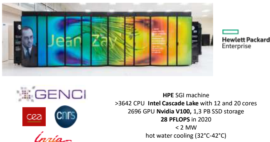
Figure 585: the Jean Zay supercomputer in France is typical of the new generation of HPCs launched since 2018 with a mix of CPUs and GPGPUs from Nvidia. Source: GENCI.
