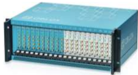
Figure 517: this Qblox system can control up to 20 qubits.
