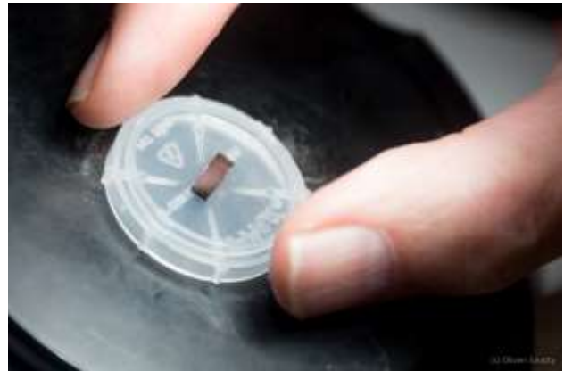
Figure 291: Daniel Esteve (CEA Quantronics) showing to the author the first operational two-transmon processor in his laboratory, June 2018.
