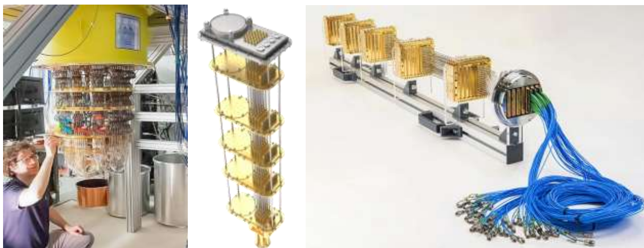
Figure 544: from left to right, Google Sycamore cable clutter, BlueFors optimized cabling system and Oxford Instrument removable cabling system. Sources: Google, Bluefors, Oxford Instruments.
