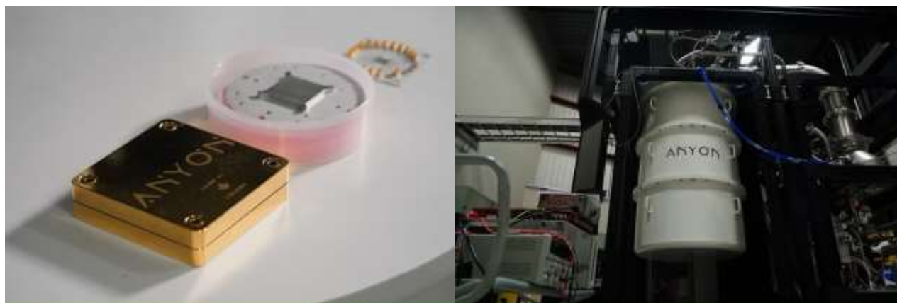
Figure 346: Anyon Systems superconducting chip and setup for its upcoming 12 qubit Monarq QPU to be delivered to Calcul Québec. Source: Quebec enters the era of quantum computing by Matthew Lapierre, CBC, August 2023.
