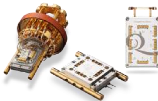
Figure 519: QDevil QCage.64 chip packaging for a superconducting qubit chip. Source: QDevil.
