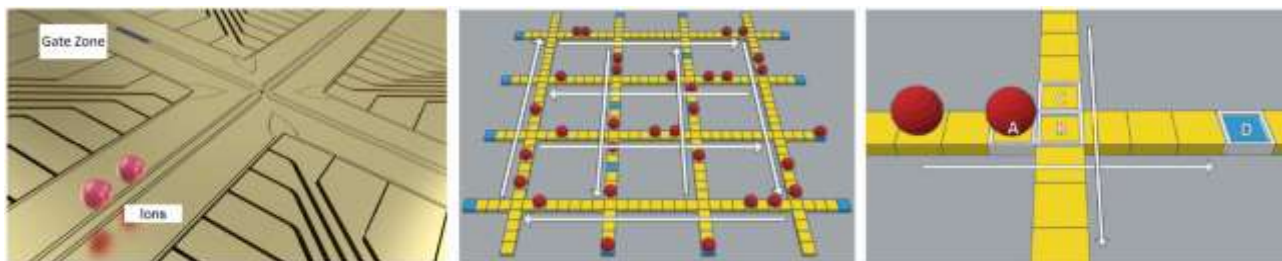
Figure 420: Universal Quantum's shuttling ion architecture in their Penning traps. Source: Universal Quantum.
