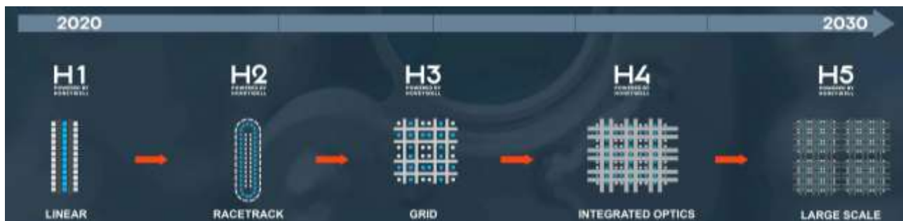
Figure 412: Quantinuum scalability roadmap. In 2023, they delivered the H2 system with a 1D race-track arrangement of qubits. Their key milestone will be to create 2D arrangement with shuttling ions, enabling larger scale quantum computing. Source: Quantinuum. 2023.
