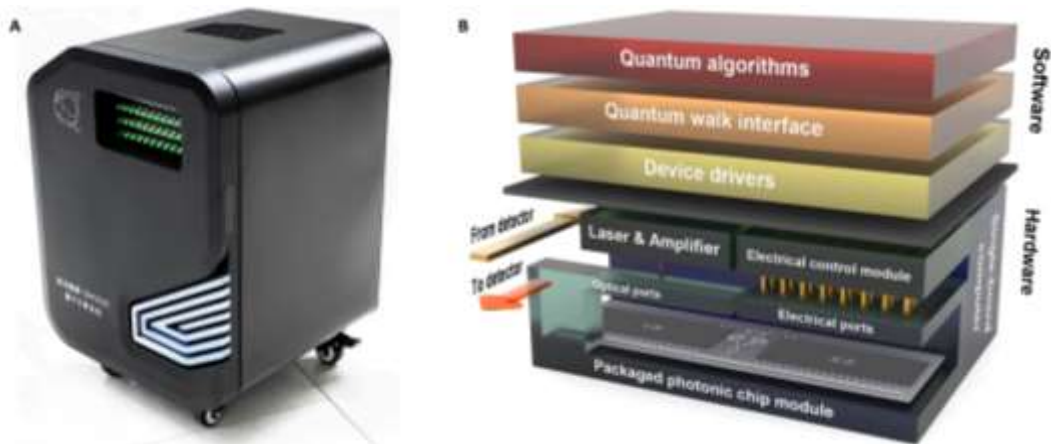
Figure 452: the continuous-variable quantum walk system YH QUANTA QW2020 from China. Source: Large-scale full-programmable quantum walk and its applications by Yizhi Wang et al, August 2022 (73 pages).
