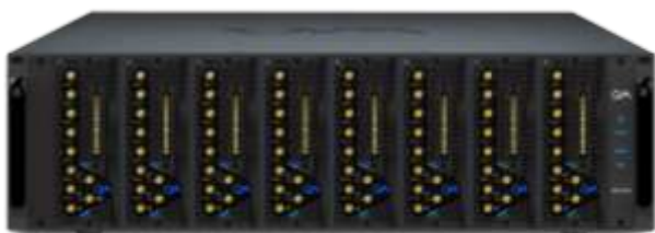
Figure 518: OPX1000 is a full-stack solution for qubit control and measurement, enabling closed-loop error correction with 64 output line for qubit control and 16 input lines for qubit readout, spread in 8 modules, and packed in a 3U rack. Source: Quantum Machines. 2023.
