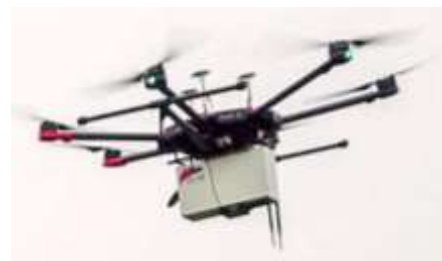
Figure 714: an airborne LIDAR to detect gas leaks.
