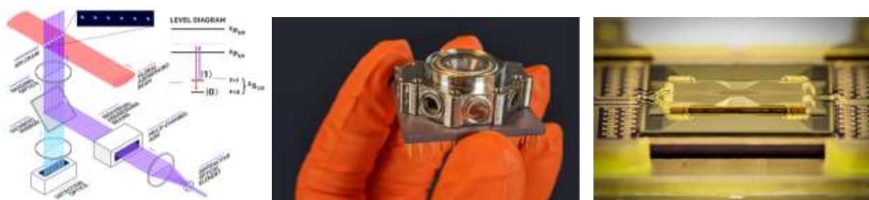
Figure 408: IonQ trapped ion drive system, the small vacuum enclosure where the ions are located, and the chip controlling the ions position coming from the DoE's Sandia Labs. Sources: IonQ and Ground-state energy estimation of the water molecule on a trapped ion quantum by Yunseong Nam, Christopher Monroe et al, March 2019 (14 pages).
