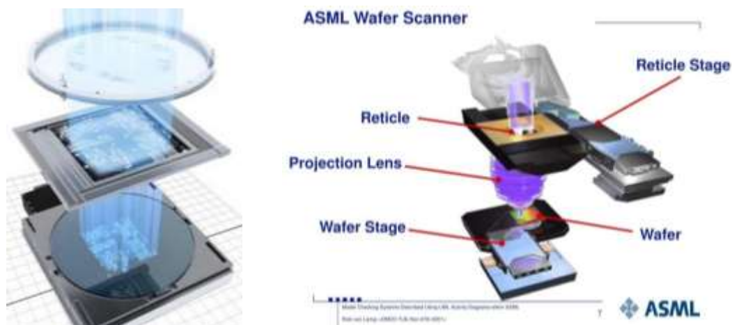
Figure 13: reticle used in photolithography and its related optics, explaining the size limitation of dies in semiconductor manufacturing.
