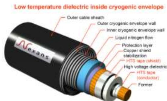
Figure 114: Nexans superconducting cable.
