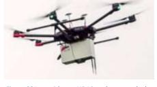
Figure 821: an airborne LIDAR to detect gas leaks.
