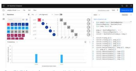
Figure 634: IBM Quantum Composer, the graphical tool to design your quantum circuit, interacting with the language version on the left. Source: IBM Quantum Experience.
