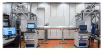
Figure 770 above and below, ETH Zurich 5 meter cryogenic microwave link. Source: <u>Microwave Quantum Link between Superconducting Circuits Housed in Spatially Separated Cryogenic Systems</u> by Paul Magnard, Alexandre Blais, Andreas Wallraff et al, PRL, December 2020 (13 pages).
