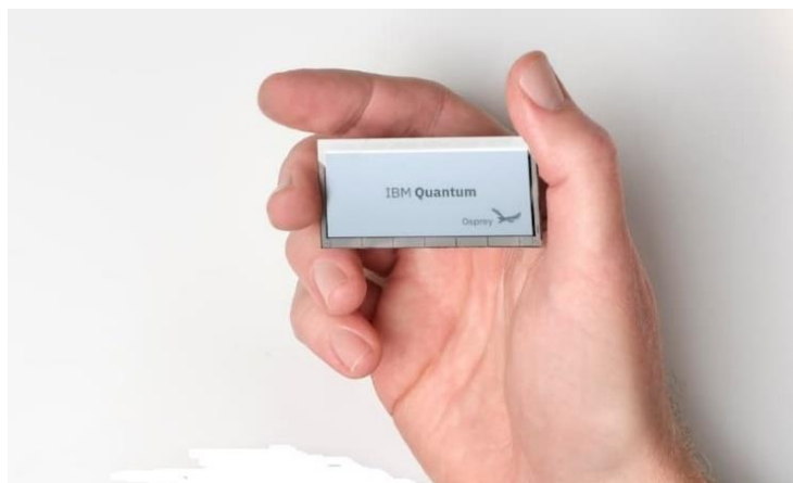
Figure 16: IBM's Osprey superconducting qubits processor shown in november 2022 and manufactured out of a 8 inch wafer. Source: IBM.
