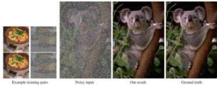
Figure 2. Random impulse noise. Our denoiser is trained on corrupted image pairs only.
