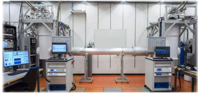
Figure 770 above and below, ETH Zurich 5 meter cryogenic microwave link. Source: Microwave Quantum Link between Superconducting Circuits Housed in Spatially Separated Cryogenic Systems by Paul Magnard, Alexandre Blais, Andreas Wallraff et al, PRL, December 2020 (13 pages).
