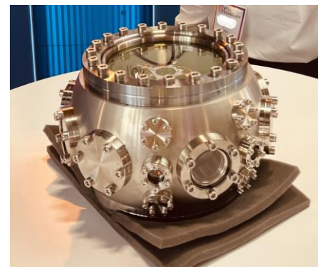
Figure 402: a vacuum chamber from Pasqal, which contains a MOT.
