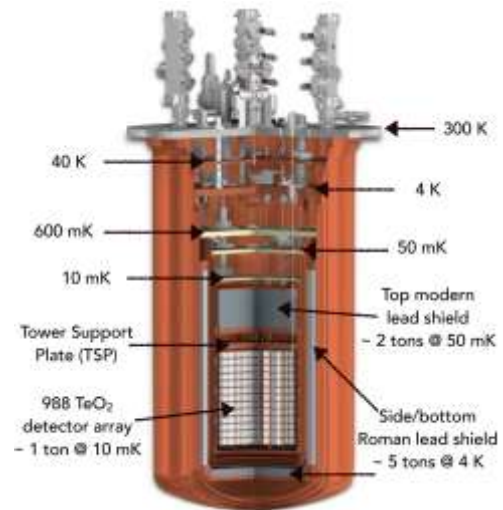
Figure 472: the CUORE mega-cryostat cooling a load of one ton.
