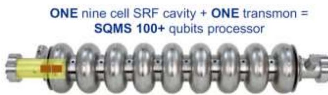
Figure 297: the huge SRF superconducting qubits from the DoE Fermilab. Source: Superconducting Quantum Materials and Systems Center by Anna Grassellino, SQMS Center Director, Fermilab, June 2021 (40 slides),
