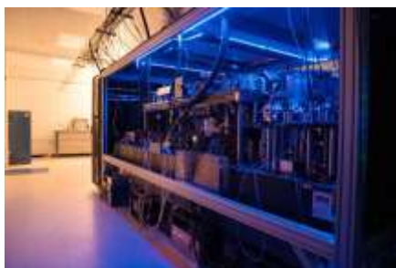
Figure 407: Atom Computing architecture for over 100-qubit gate-based computing. Source: Assembly and coherent control of a register of nuclear spin qubits by Katrina Barnes et al, August 2021 (10 pages).
