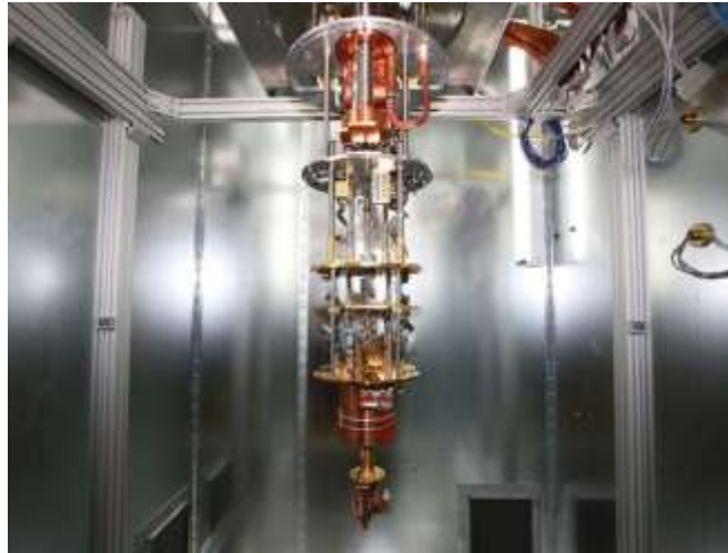
Figure 274: Inside a D-Wave system, with the cryostat open. Source: D-Wave.
