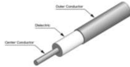
Figure 510: a typical CoaxCo niobium-titanium cable. Source: CoaxCo .
