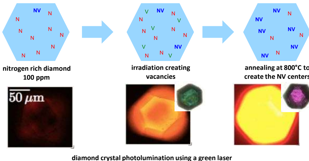
Figure 356: how are nitrogen vacancies created. Source: NV Diamond Centers from Material to Applications by Jean-François Roch, 2015 (52 slides).
