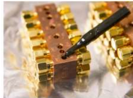
(A) ECCOSORB injection. Inject slowly and at a flat angle such that the liquid creeps onto the edge of the fill opening and into the cavity. Injecting too fast or steep will cause a planar bubble to form which blocks the opening (see Figure 3.8b).
