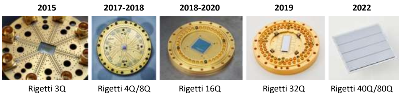
Figure 323: evolution of Rigetti actual chipsets over time. Source: Rigetti investor presentation.
