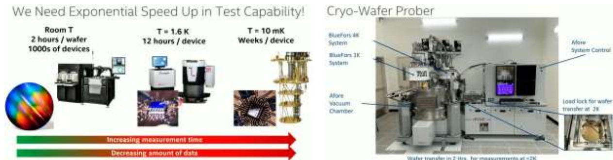
Figure 349: how Intel is saving time with a Bluefors/a-Fore cryo-prober. Source: Intel.
