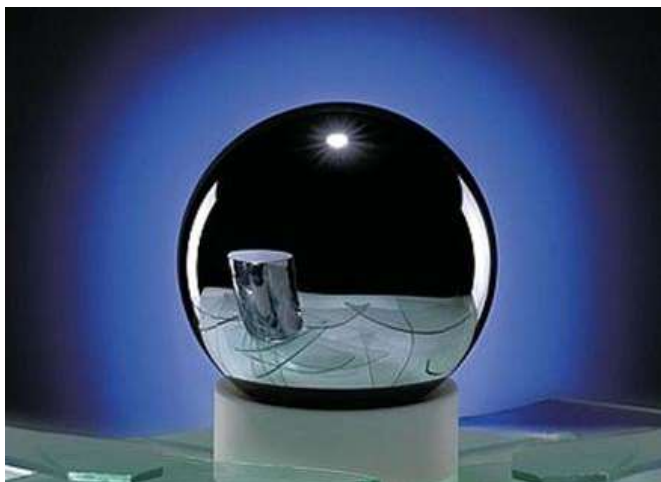
Figure 541: silicon 28 was initially produced to create a replacement for the reference kilogram used in the international metric system, as a way to determine the Avogadro number. Purifying silicon 28 was a figure of merit of this quest that is now reused in the silicon spin realm.
