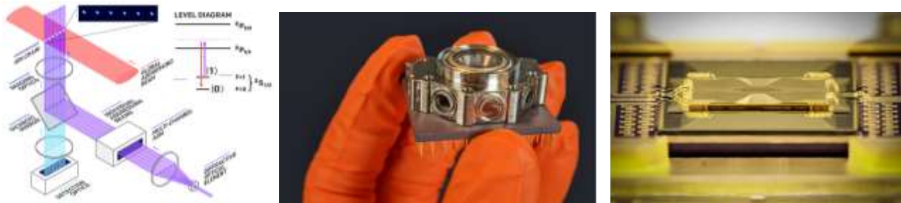
Figure 385: IonQ trapped ion drive system, the small vacuum enclosure where the ions are located, and the chipset controlling the ions position. Sources: IonQ and Ground-state energy estimation of the water molecule on a trapped ion quantum by Yunseong Nam, Christopher Monroe et al, March 2019 (14 pages).
