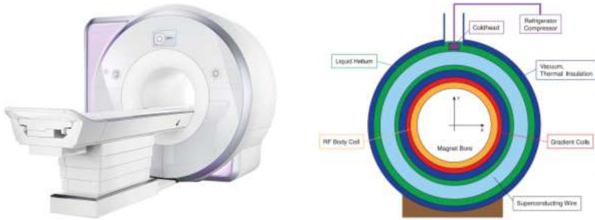
Figure 102: MRI principle. Source of illustration on the right: Helium Reclaiming Magnetic Resonance Imagers by Dan Hazen, MKS Instruments (5 pages).
