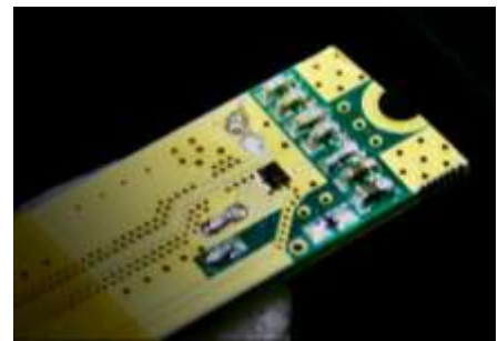
Figure 354: Archer-EPFL spin-resonance circuit. Source: Archer.
