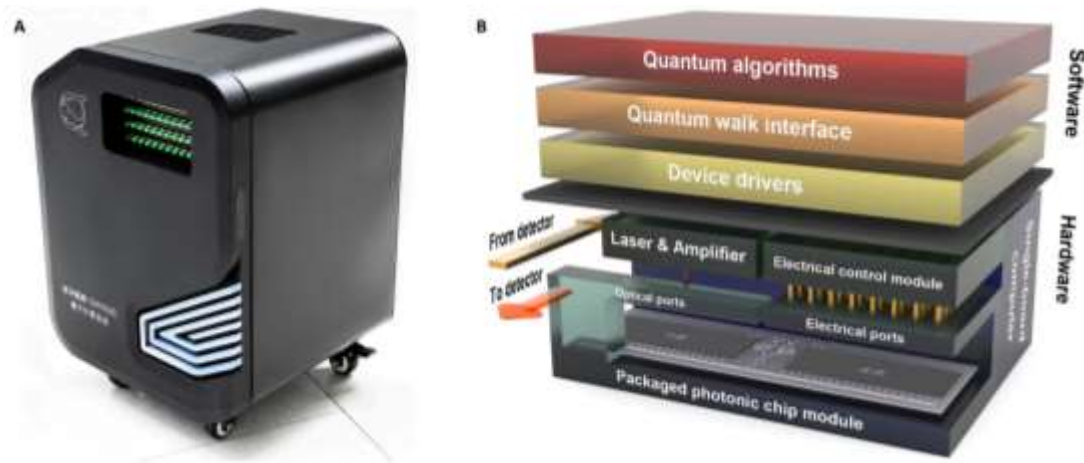
Figure 425: the continuous-variable quantum walk system YH QUANTA QW2020 from China. Source: Large-scale full-programmable quantum walk and its applications by Yizhi Wang et al, August 2022 (73 pages).
