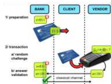
Figure 1. Practical quantum money protocol. The sequence of interactions between the credit card holder (client), the bank and the vendor involved in the transaction. In the preparation phase, the bank uses a secret key to prepare the quantum state loaded on the credit card, which is then given to the client. In the transaction phase, the vendor randomly selects one out of two challenge questions, measures the qubits and sends the outcome to the bank, who can then verify the validity of the credit card or detect a forgery attempt.
