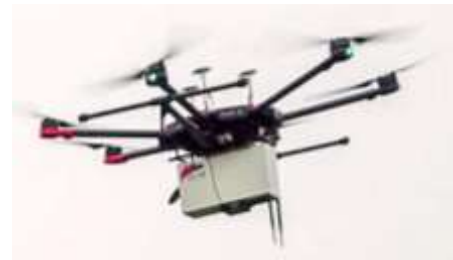
Figure 821: an airborne LIDAR to detect gas leaks.
