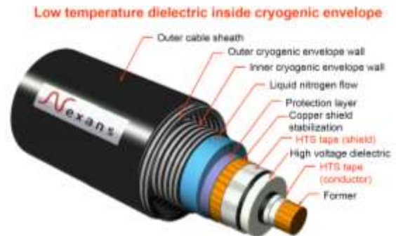
Figure 103: Nexans superconducting cable.
