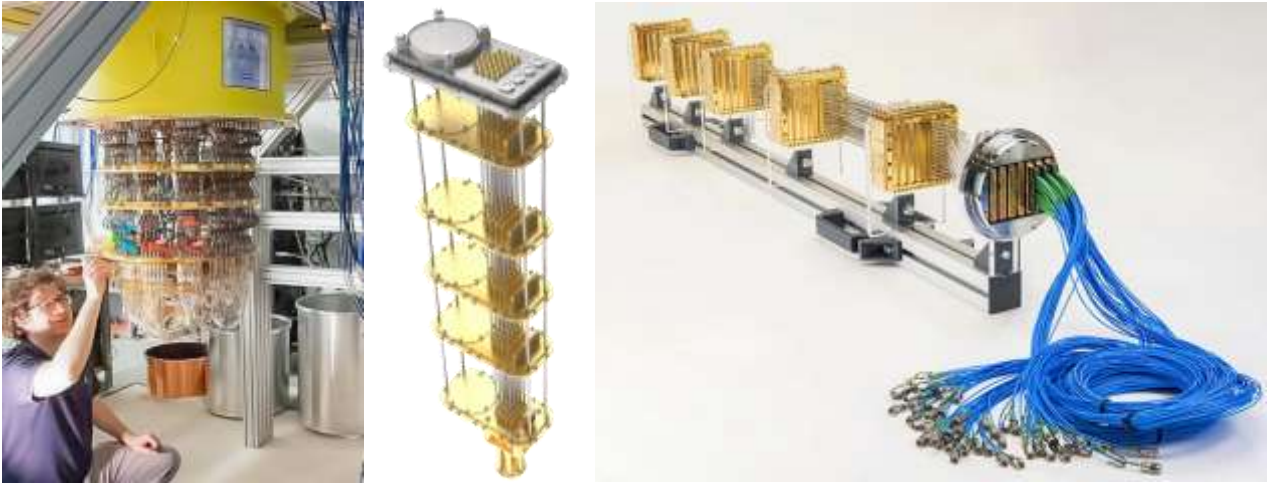
Figure 511: from left to right, Google Sycamore cable clutter, BlueFors optimized cabling system and Oxford Instrument removable cabling system. Sources: Google, Bluefors, Oxford Instruments.
