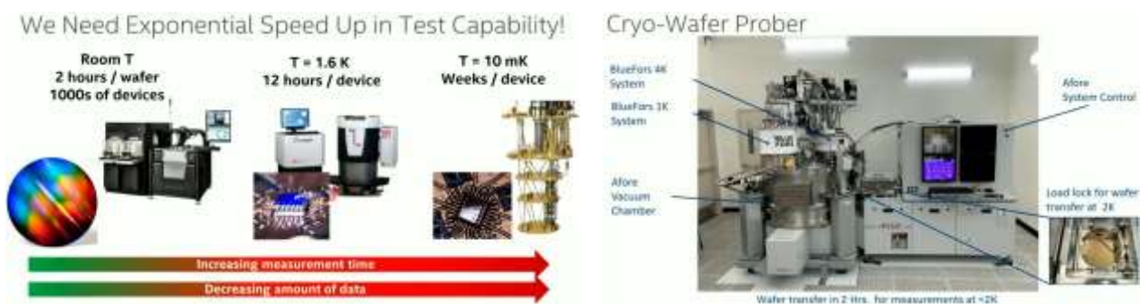
Figure 349: how Intel is saving time with a Bluefors/a-Fore cryo-prober. Source: Intel.
