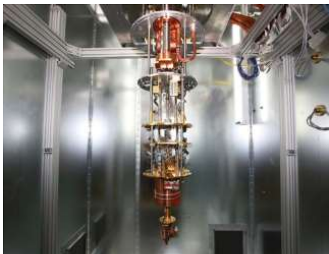
Figure 274: Inside a D-Wave system, with the cryostat open. Source: D-Wave.
