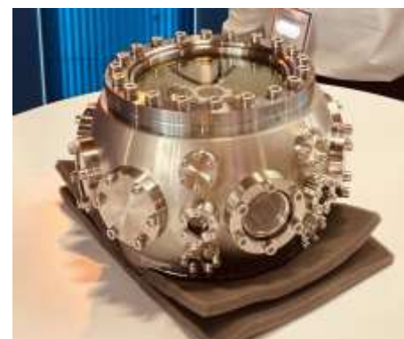
Figure 402: a vacuum chamber from Pasqal, which contains a MOT.
