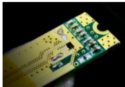
Figure 354: Archer-EPFL spin-resonance circuit. Source: Archer.
