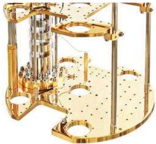
Figure 466: cold plate with a gold finish which is used to facilitate the assembly with experimental devices and optimize thermal conductivity. Photo: Bluefors.
