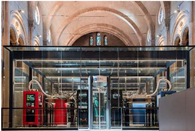
Figure 37: The Marenostrum Qilimanjaro quantum computer with 10 qubits, to be upgraded later with more qubits. It sits in a chapel at the Barcelona Supercomputing Center. Source: Qilimanjaro [334].
