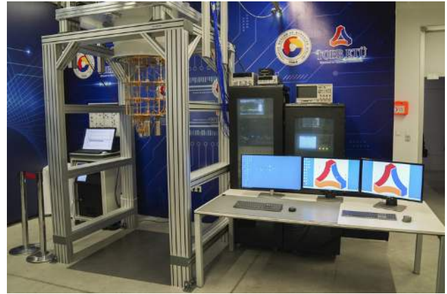
Figure 42: TOBB 5-qubit superconducting QPU presented in 2024.
