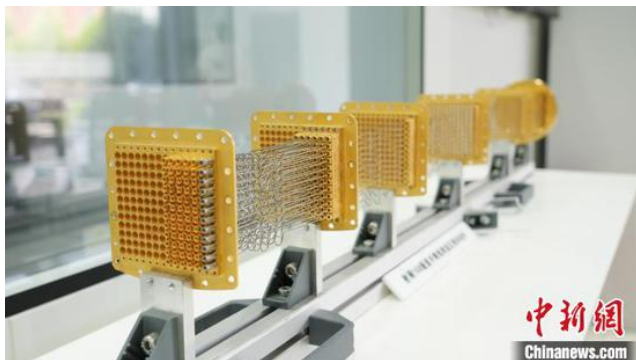
Figure 48: Origin Quantum high-density microwave system looks like equivalent you can find with Bluefors and Oxford Instruments.
