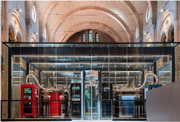
Figure 37: The MareNostrium Qilimanjaro quantum computer with 10 qubits, to be upgraded later with more qubits. It sits in a chapel at the Barcelona Supercomputing Center. Source: Qilimanjaro [334].
