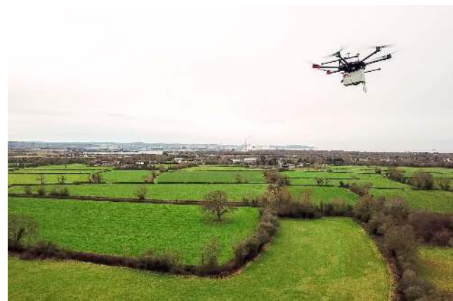
Figure 160: An airborne LiDAR to detect gas leaks.
