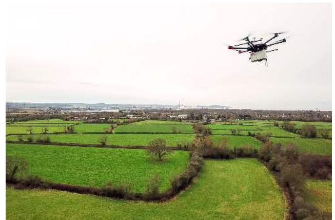
Figure 158: An airborne LiDAR to detect gas leaks.
