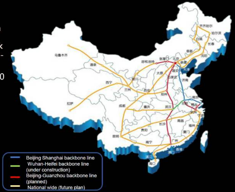
Figure 45: China's 33,000 km QKD backbone plan as presented in 2019. The operational CN-QCN reported in 2025 contains approximately 10,103 km of newly deployed backbone fiber, interconnected with the earlier Beijing-Shanghai backbone and metropolitan networks [282].
