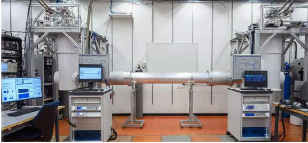
Figure 66: ETH Zurich 5-meter cryogenic microwave link. The waveguides were cooled to below 20 mK. Source: [812].
