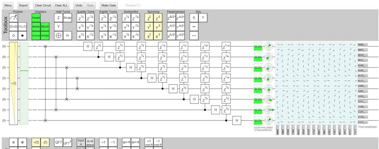
Figure 93: Quirk, an open-source visual quantum-programming tool that runs in a browser and supports up to 16 qubits in vector-state mode. It runs on a laptop and even a smartphone. It was developed by Craig Gidney before he joined Google. Source: Quirk Algassert.
