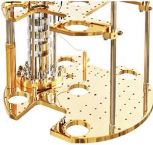
Figure 347: Cold plate with a gold finish which is used to facilitate the assembly with experimental devices and optimize thermal conductivity. Photo: Bluefors.
