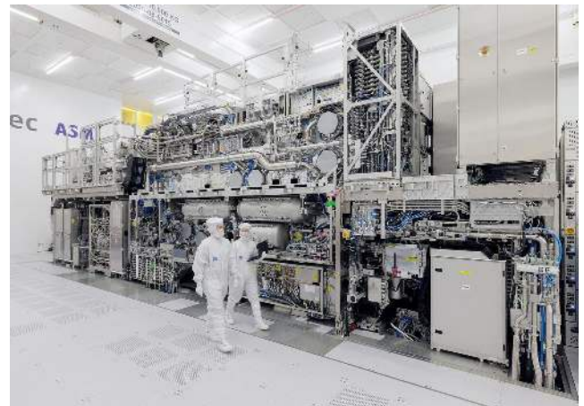
Figure 444: A typical ASML EUV photolithography system, without its doors. Probably a TWINSCAN EXE:5200B. Low-NA (0.33) EUV systems resolve down to 13 nm while this High-NA machine reaches 8 nm single-exposure resolution with 0.7 nm overlay, thanks to its 0.55 NA (numerical aperture) anamorphic projection optics, both at the same 13.5 nm wavelength. Source: ASML.
