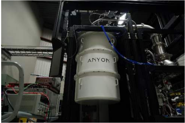
Figure 93: Anyon Systems superconducting setup for its 12 qubit Monarq QPU that was delivered to Calcul Québec. Source: [1177].
