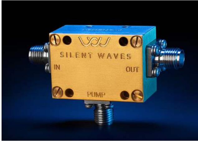
Figure 412: Silent Waves's ZEPHYR TWPA in its packaging, including a pump coupler. Source: Silent Waves. 2026.
