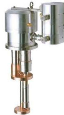
Figure 350: A Bluefors/Cryomech PT420 pulse tube, that cools a cryostat down to 4 K. Its cooling power is of 2 W at 4.2 K and 55 W at the 45 K stage. Indeed, these pulse tubes have two stages that are visible in the pictures, being attached to two consecutive cold plates in the cryostat. The pulse tube is also used to cool down the helium 3 and 4 mixture circulating in a dilution that is attached to the pulse tube. Source: Bluefors.
