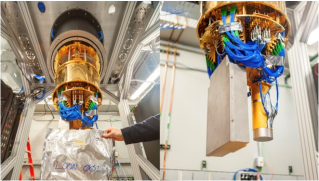
Figure 55: IBM Loon experimental cryostat in 2026. The grey box contain the readout circulators and TWPAs while the cylinder contains the superconducting chip. Source: IBM.
