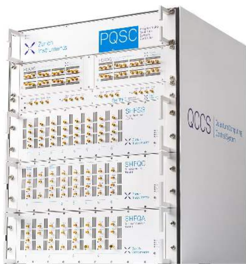
Figure 384: Zurich Instruments QCCS containing a PQSC (program and control), two HDAWG (arbitrary waves generators) and three SHFQC (signal generators and readout) and one SHFPPC (tone pulse for parametric amplifier) for qubit control and readout.
