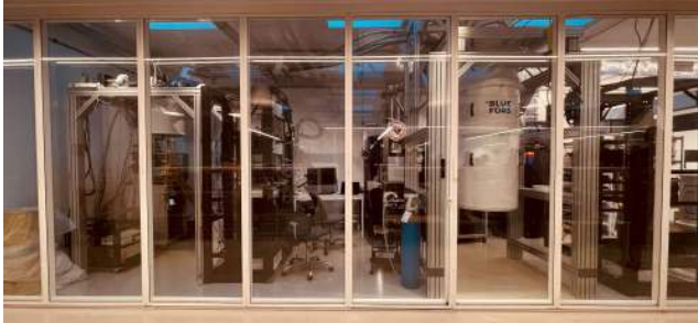
Figure 150: C12's testing room with two cryostats, a typical setup for many quantum computing startups nowadays. They have two other floors for their carbon nanotube and related circuits manufacturing tooling. © Photo: Olivier Ezratty, 2023.
