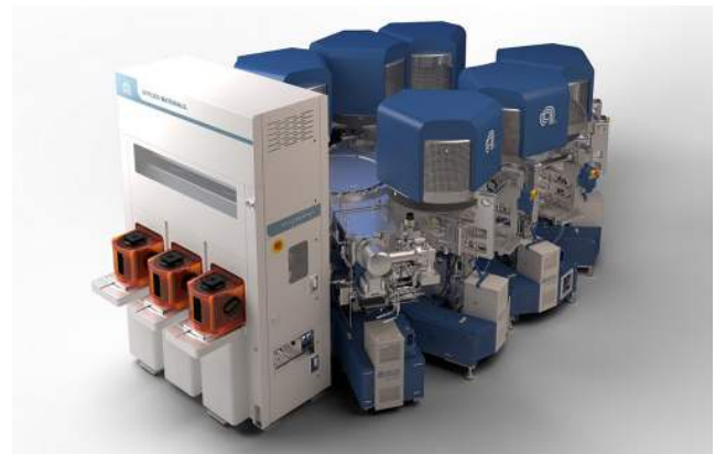
Figure 447: Applied Materials Endura Clover MRAM PVD System ( source ).
