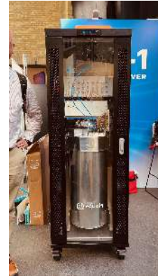
Figure 137: equal1 Bell-1 integrated QPU with its integrated cooler that reaches 300 mK for supporting their qubit chip operating temperature. Photo: Olivier Ezratty, May 2025 in Amsterdam at Q-Expo.
