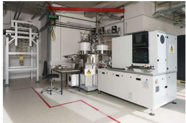
Figure 135: Quobly cryo-prober from aFore-Bluefors that speeds up their characterization of a full chip wafer. Source: Quobly, 2025.
