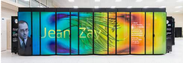
Figure 472: The Jean Zay supercomputer in France is typical of the new generation of HPCs launched since 2018 with a mix of CPUs and GPGPUs from Nvidia. This mid-size supercomputer is built by HPE. It hosts 3,642 CPUs from Intel, 2,696 Nvidia V100 GPU, 1.3 PB of storage, had a peak power of 28 PFLOPS in 2020. It was cooled with hot water (32°C-42°C). Source: GENCI.
