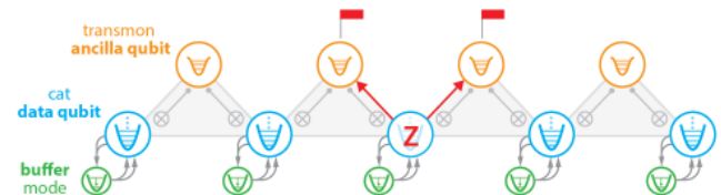
Figure 106: The first publicized cat-qubit chip from AWS. Ocelot uses five bosonic cat-qubit data modes and four transmon ancillas forming a single distance-5 repetition code. Intrinsic cat stabilization suppresses bit flips, while repeated syndrome measurements correct residual phase flips. Source: [506].
