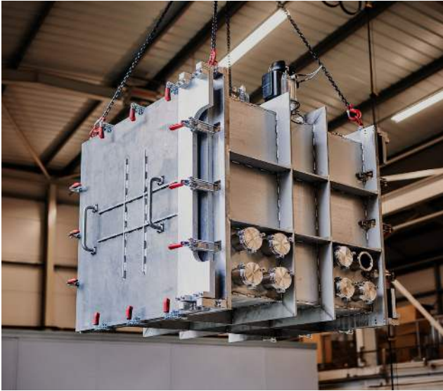
Figure 312: PsiCube, the first PsiQuantum prototype cabinet cooled with liquid helium with a cooling power of 10W at 2.3K.
