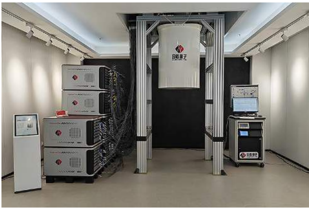
Figure 42: A rare glimpse on a China Zuchongzhi 2.1 QPU in 2023. Source: [845].
