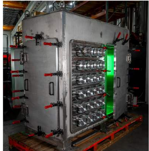
Figure 313: PsiQuantum prototype Mk2 cabinet hosting 100 Omega chips and cooled with liquid helium with a cooling power of about 50W at 2.3K.
