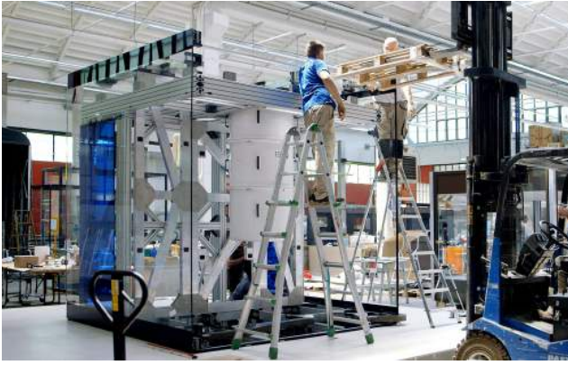
Figure 44: IBM System One during assembly. The white cylinder corresponds to the casing hosting the Bluefors XLD dilution refrigerator. The whole system contains the whole compressor and gas-handling system supplying the dilution refrigerator with helium 3 and 4, as well as all control electronics. Source: IBM.
