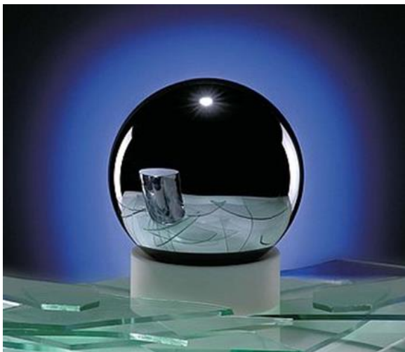
Figure 461: ^{28}\text{Si} was initially produced to create a replacement for the reference kilogram used in the international metric system, as a way to determine the Avogadro number. Source: PTB, 2010 in [3515].
