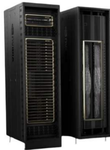
Figure 17: A Nvidia NVL72 rack with its 72 GPUs and 36 CPUs. Source: Nvidia.
