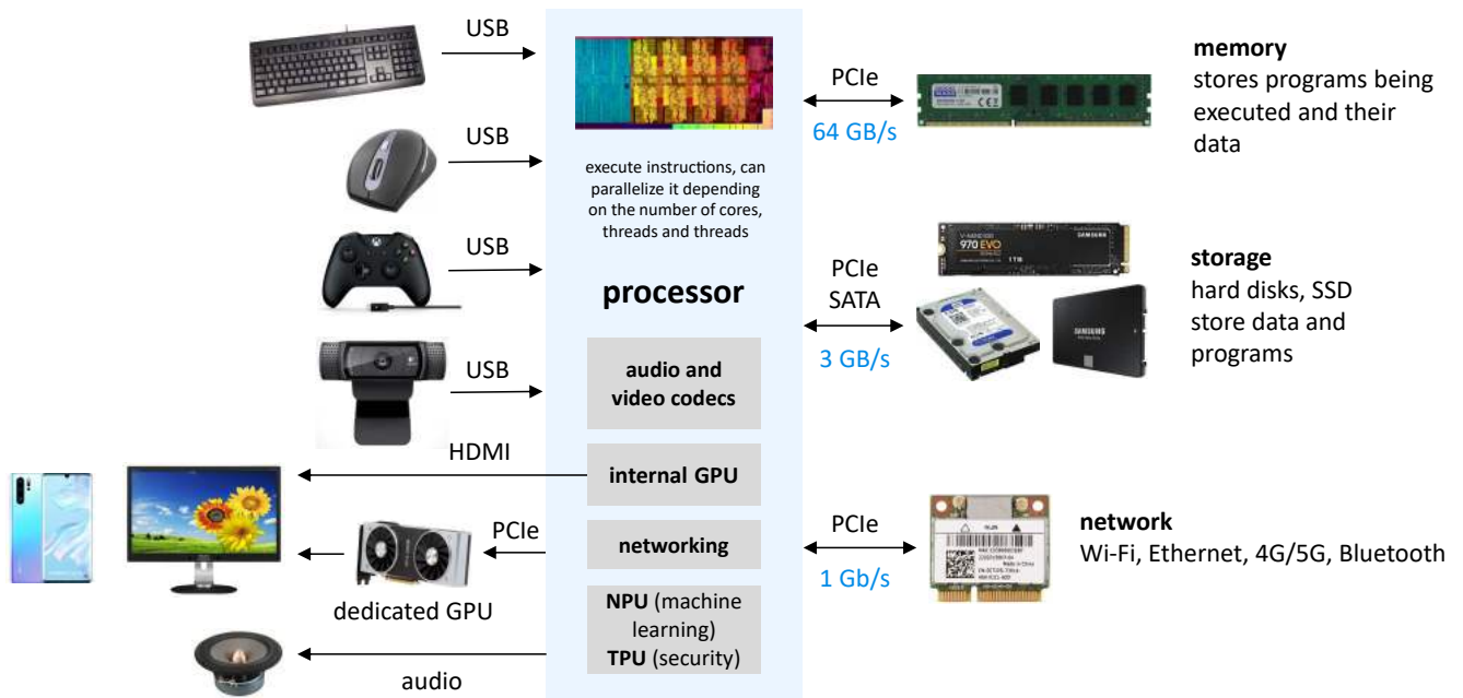
Figure 230: Illustrative personal computer hardware architecture, shown as a familiar baseline rather than as a complete model of contemporary classical computing. It leaves aside accelerators, the full memory hierarchy, high-speed interconnects and the distributed system features that matter when a quantum computer is integrated in a data center. © Olivier Ezratty, 2021-2024.
