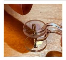
See Non-classical correlations between phonons and photons in a MHz-frequency mechanical oscillator coupled to an optical cavity by Ivan Galinskiy, Georg Enzian, Micha? Parniak and Eugene Polzik, December 2023 (6 pages). Below are the filter cavities used in the experiment.
