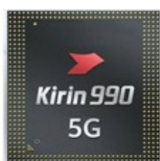
Kirin 970 / 980 / 990 NPU 10 / 7 nm 2-4 TOPS Huawei Mate 10, Pmate 20, Honor 10, (K970), Honor View 20, Huawei Mate 20, Mate X (K980)
