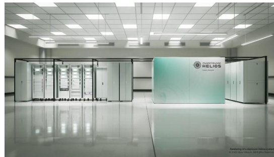
Quantum Helios, 98 qubits, 34 kW, uses liquid helium cooling
