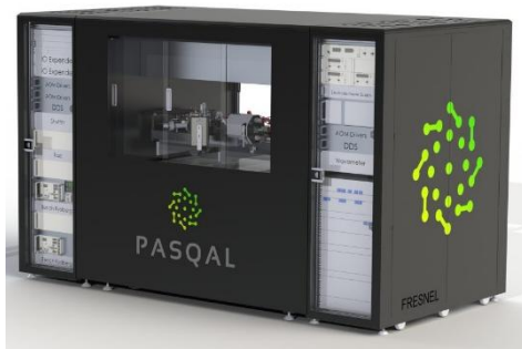
Pasqal Orion Gamma, >140 qubits in analog mode, 3 kW
