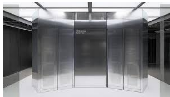
IBM System Two < 150 kW, hosting three 156-qubit Heron processors
