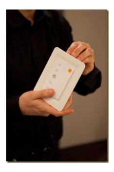
• The **Tabbee**, a tablet positioned as a secondary home TV, bathroom tablet, digital picture frame. Uses Wifi to connect to DSL broadband router. Built by Sagem and using Linux and some internal (?) middleware. It's shipped for 250 Euros with a couple applications including "Cookineo" for getting cooking recipes. Cookinero is a service built by Domolib, a Parisian startup incubated by Agoranov.
